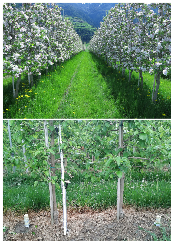
FIGURE 2 Upper photo: Apple tree rows in the right field in April 2015. Lower photo: Tension lysimeters (at 25 cm on the left hand, at 50 cm on the right hand) and wires connected to the buried soil moisture probes
