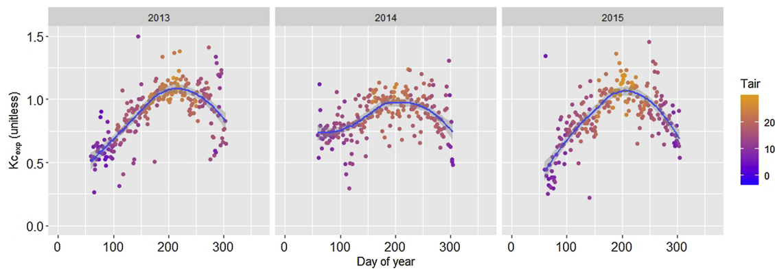
Fig. 5. Daily values of K_c ( K_{c_{exp}} ) over the vegetative period (March–October) of three years. The colour of the dots reflects the mean daily air temperature. The trend-line for each year (presented with 95% confidence interval – grey area around the line) is obtained by the loess non-parametric regression method with the default span of 0.75.
